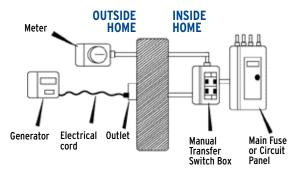
Have an electrician install a transfer switch to prevent backfeed. This is the safest way to hook up a portable generator.
