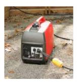
If you are unable to find a wattage label, you can compute the running wattage of an appliance by multiplying its AMPS by its VOLTS. Remember, motor-driven appliances (refrigerators, freezers, air conditioners, furnace blowers) require up to three to ten times their normal wattage to start or to periodically cycle a compressor.
